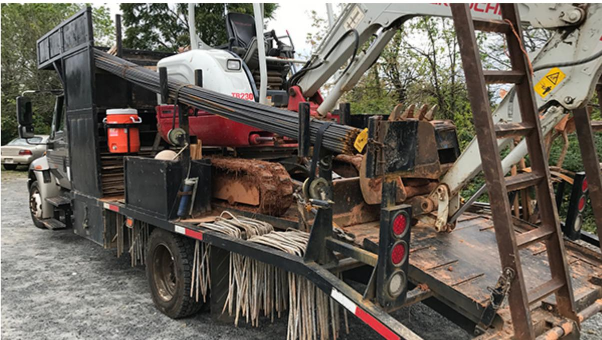
of the many interesting things I saw there was how they carried their rebar on their trucks. They had tilted their rebar racks downwards towards the rear of the truck. Instead of placing the rebar on top of a tall, level truck rack, this angled rack was a simple stroke of genius.
